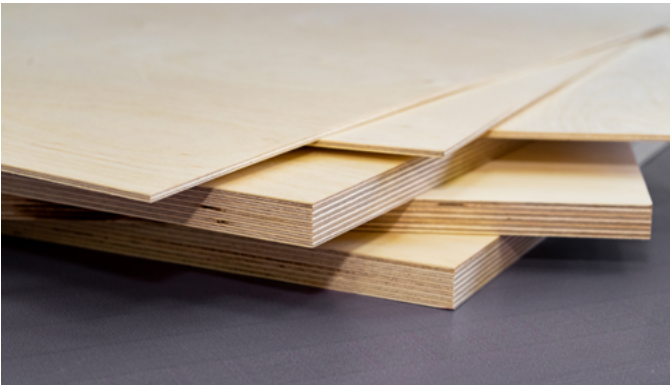
Fig. 3: Engineered wood that uses multiple layers of thin wood assembled with adhesives. Often in combination with wood frame
