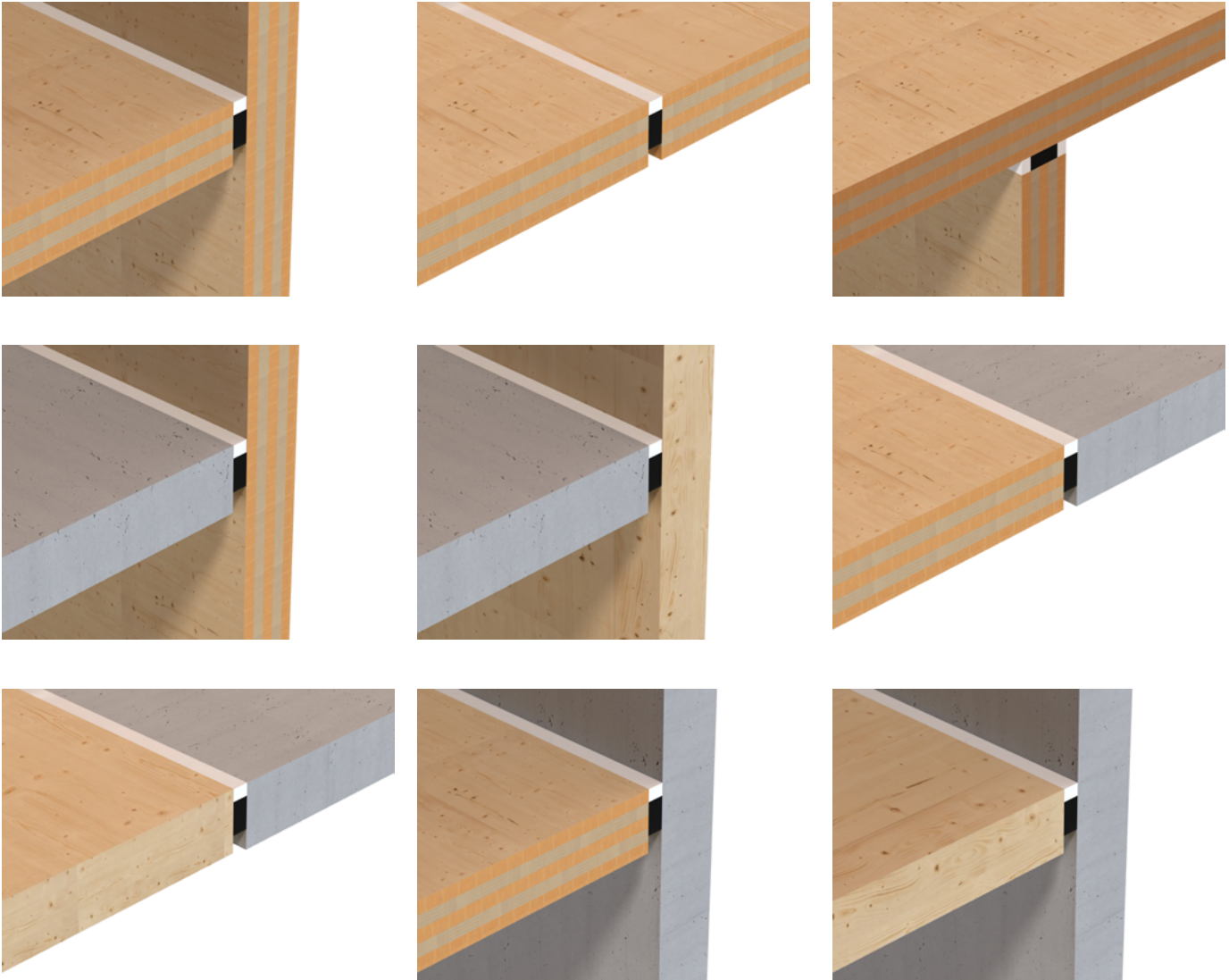
Fig. 8: Some of the most common fire-rated joint types in buildings with wood elements.
