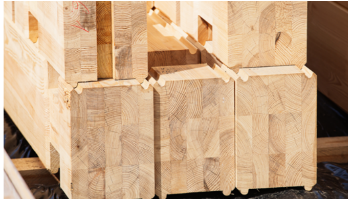
Fig. 2: Engineered wood that has perpendicular wood laminates glued together
