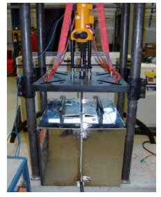
Tension cylinder on the furnace
