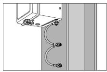
Protective bonding circuit – Double point connection
