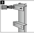
Drive **X-BT** studs with **DX 351 BT** tool and **X-BT** cartridge.
