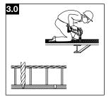
Pre-drill with **TX-BT 4/7** step shank drill bit.
