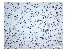
**Figure 3.** Micro section of cast iron EN-GJS-400-18LT: Spheroidal graphite embedded in ferritic matrix
