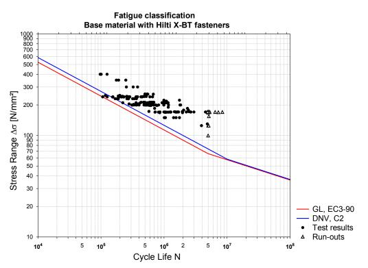
Figure 2. Test data compared with approved GL and DNV fatigue categories
