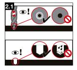
Pre-drill until shoulder grinds a shiny ring. The drill hole and the area around drilled hole must be clean and free from liquids and debris.
