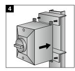
Position unit on studs and hold in place. Fit washers and start tightening by hand to avoid cross threading.
