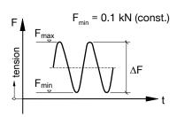
Figure 4. Principle sketch of cyclic tension tests
