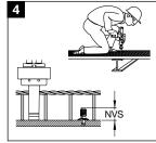
Drive fastener only with **DX 351 BT G** tool and 6.8/11M brown cartridge.
