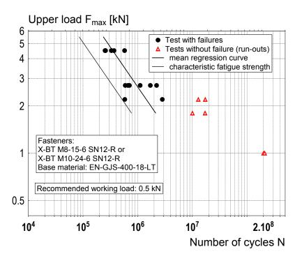
Figure 6. Results of cyclic tension tests
