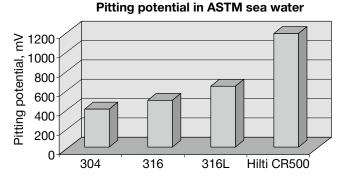
Potential-static test carried out with rods and nails in synthetic sea water as per ASTM D 1141
