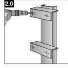
Pre-drill with **TX-BT 4/7** step shank drill bit.
