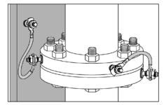
Functional and protective bonding in pipe (Outer diameter of installed surface ≥ 150mm)
