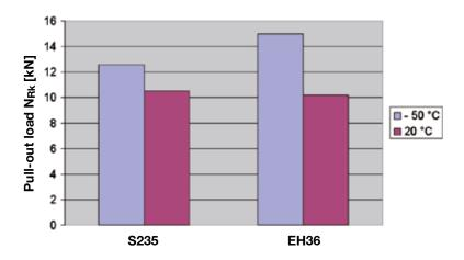
At low temperature the pull-out resistance is increasing compared to that at room temperature.
