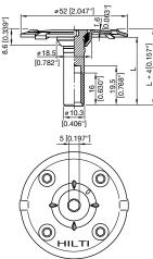
Important: The X-FCM-R system is not designed or intended to resist shear loads.
