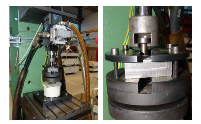
Figure 5. Servo-hydraulic test setup for tension fatigue tests
