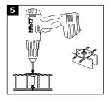
Tighten **X-FCM-R** with 5 mm Allen-type bit.
