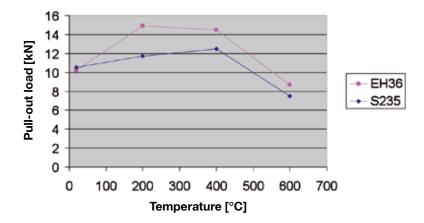
At 600°C, the pull-out resistance of the X-BT has about 71% of its 20°C strength left in steel S235 and about 85% in steel EH36.
