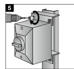
Tighten using a screwdriver with torque clutch.
